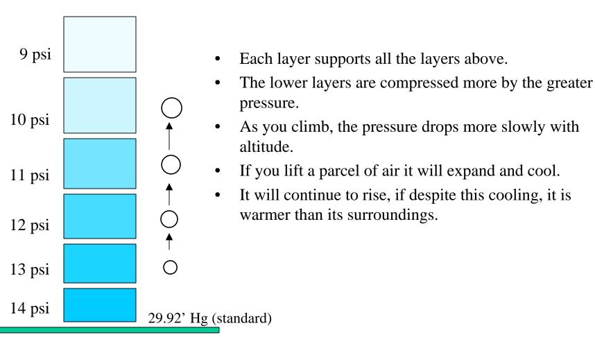
The atmosphere becomes unstable if the temperature drops sufficiently rapidly with altitude
