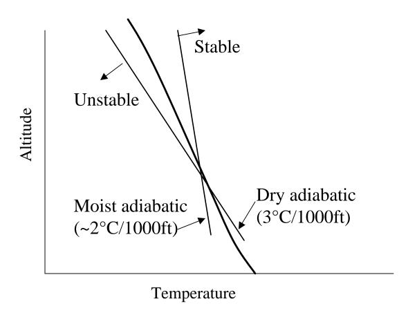
Conditional instability when the ambient lapse rate lies between the dry and moist rates. The air is then unstable if it is/becomes saturated.
