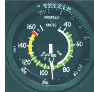
Lift (and drag) are proportional to  $\text{air\_density} * \text{TAS}^2$  i.e  $\rho v^2$
