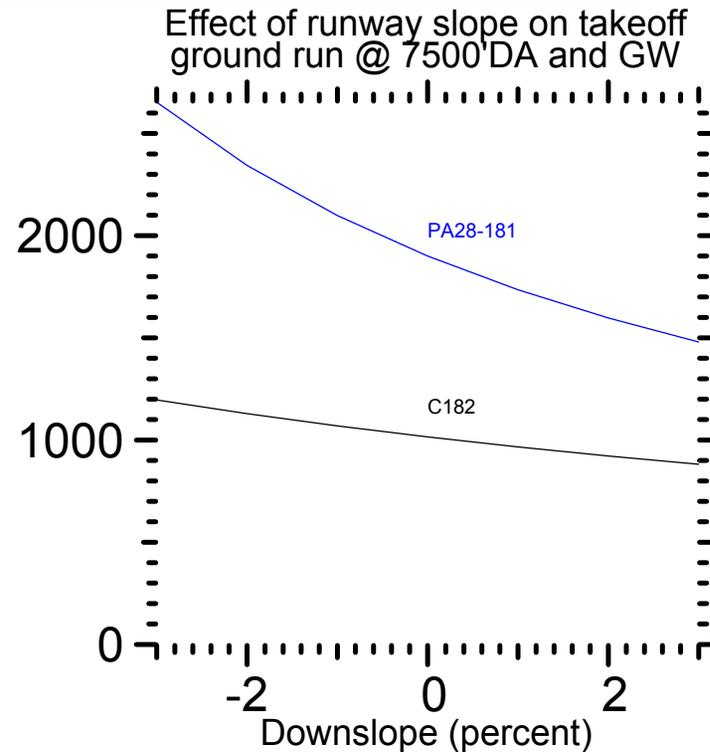
*Ground roll decreases about 6% per thousand feet of ground roll for each percent of downslope. (Same **increase** for landing ground roll.)*
