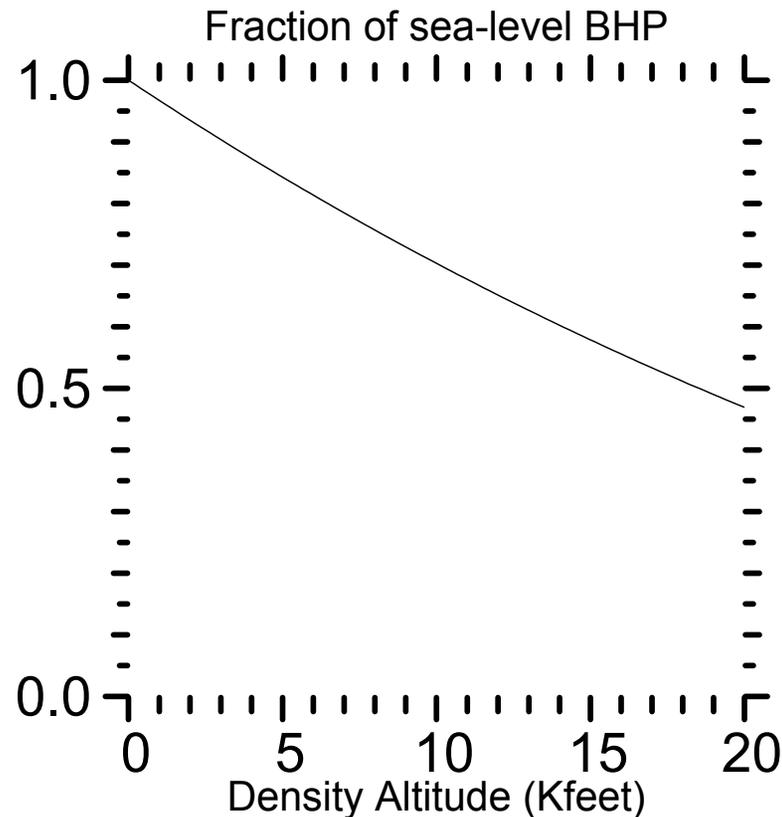
The minimum power required for level flight increases with altitude. (The minimum drag doesn't change – but you have to fly faster.)
